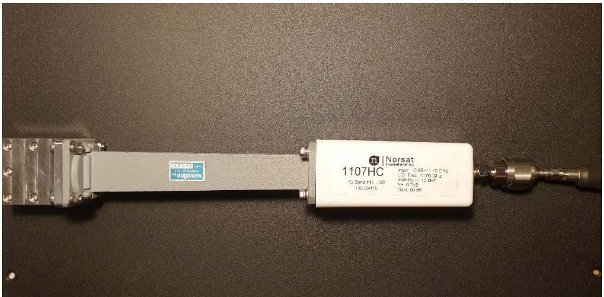
Fig. 3 – Measurement setup with the LNB NORSAT 1107HC
